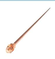
The copper cladded earth spike or stake is used to earth the electric fence system. A minimum of 3 earth spikes must be knock into the ground near the electric fence at a minimum of 1.2m apart. Connect these earth spikes to the energizer or the fence using the high tension insulated cable (HT). In areas where earthing conditions are bad you may be required to add a few more earth spikes/stakes along the fence line and connect these back to the energiser.
