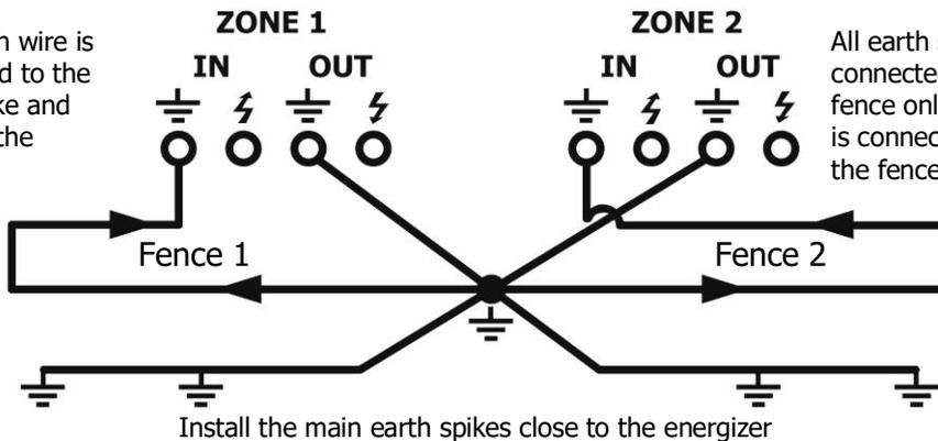
All earth spikes are connected to one wire of the fence only, and this one wire is connected to the rest of the fence at the main.
