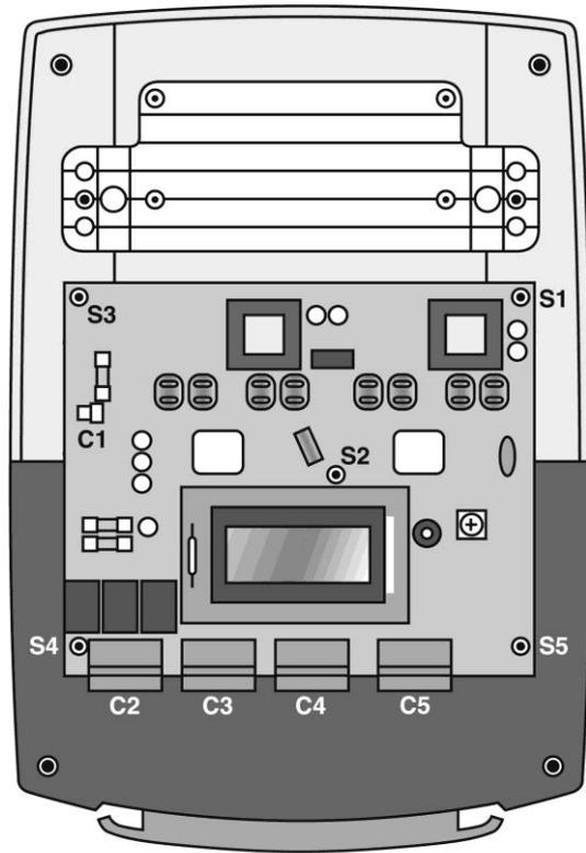
**STEP 5:** To replace the PC Board, first align the box connector near the bottom of the PC Board and then align the four spade connectors at the top of the PC Board using the guide tabs, and gently press the PCB down into place.
