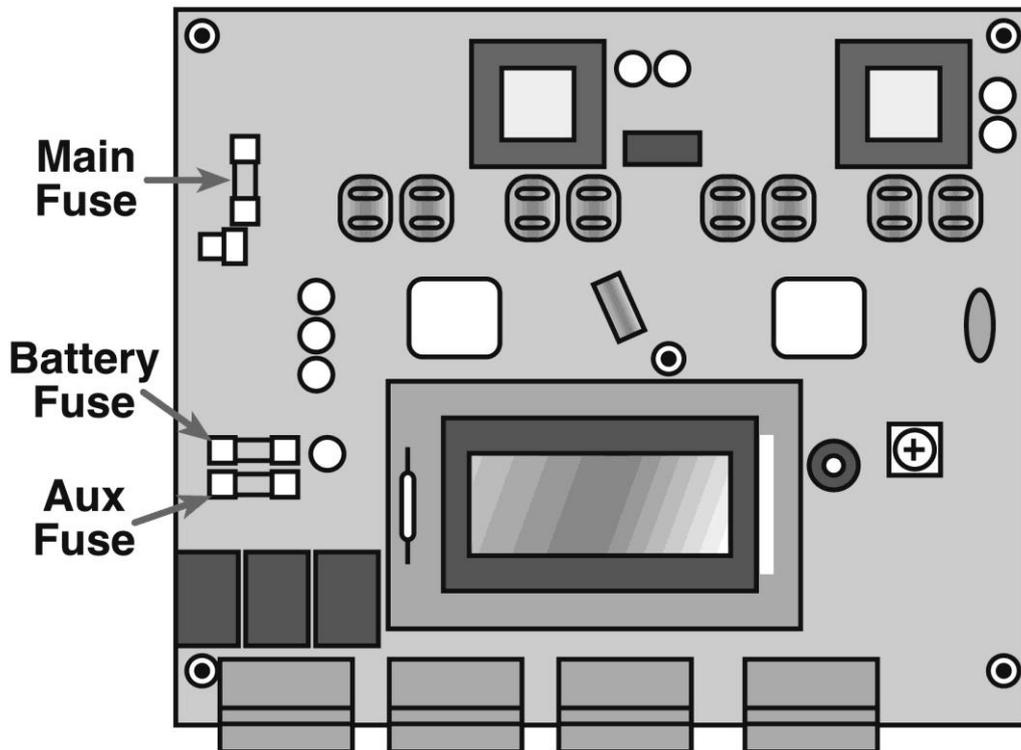
**Main Fuse:** Energizer displays a battery symbol, and not the mains power symbol (plug).
