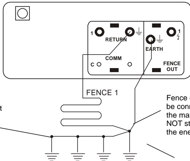
The earth spikes are connected to one wire of the fence and the wire is only coupled to the other fence earth wires at the main earth spike
