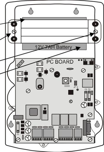
**STEP 4:** Drill 4 x 8mm holes for mounting the unit. Four nail-in anchors are supplied with the unit. Insert the plastic sleeve of the nail-in anchor from the inside of the box and then hammer the screw in with a screw driver and hammer.
