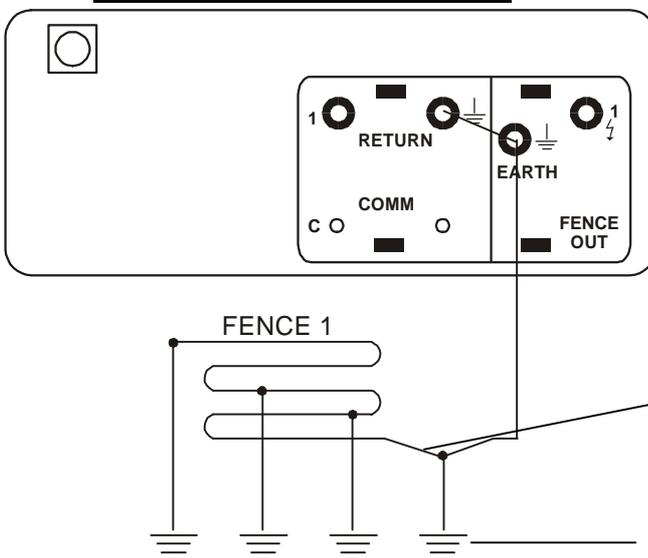
Fence earth wire to be connected from the main earth spike, NOT straight from the energizer
