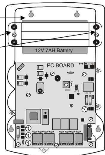
**STEP 6:** Place the battery bracket back and fasten the screws.
