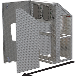
Slide out the battery cover
